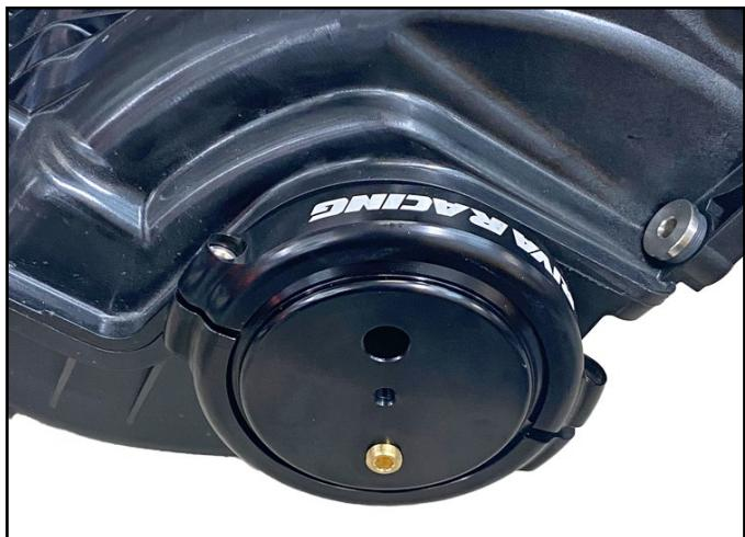
Place one half of the block-off clamp with RIVA logo on top of the block-off insert. Place other half of block-off clamp with 3 cut outs onto bottom of block-off insert so the cut outs are against the intake manifold.
