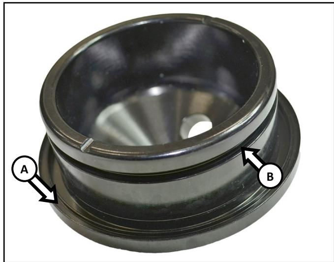
Apply a liberal coating of waterproof grease onto supplied o-ring that is smaller in diameter. Place o-ring onto block-off and into groove B.
