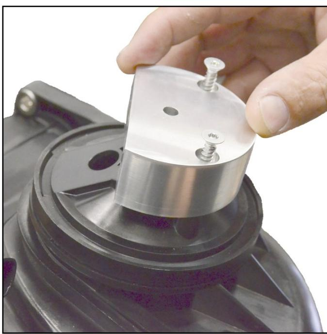
Fasten drill bit guide to intake manifold with supplied flat self-tapping screws (2).
